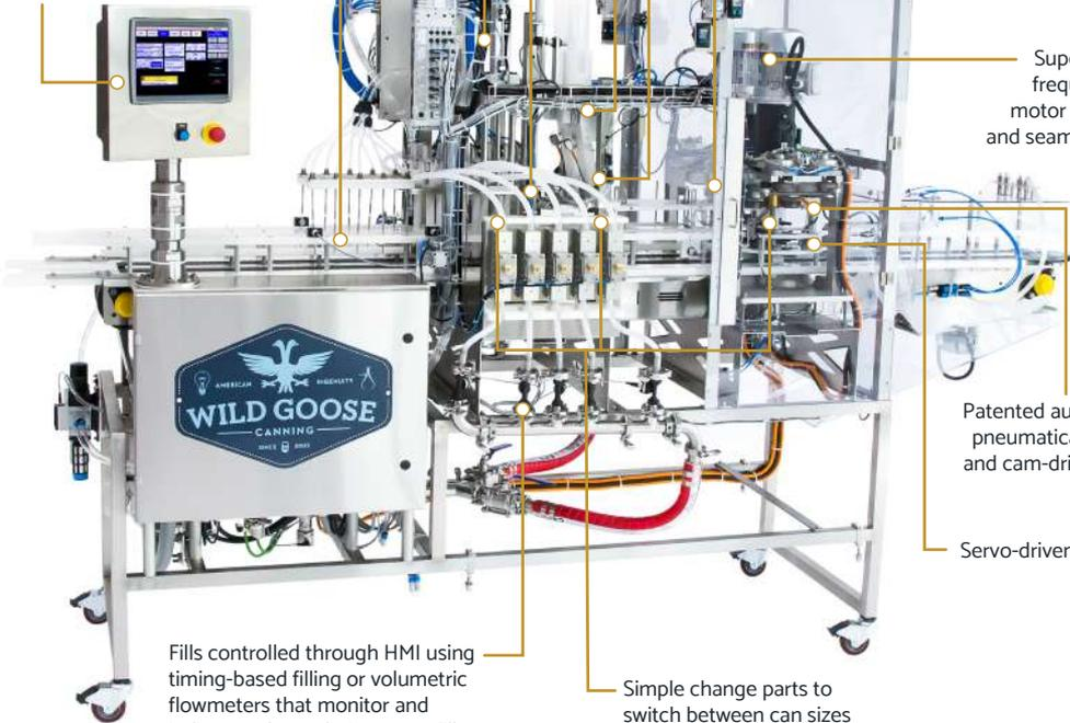
Patented automatic dual pneumatically-actuated and cam-driven seamers
