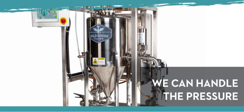
For a smooth filling process, it is important to regulate high fluid pressure coming from your product tank and transfer hose into your filling system. Wild Goose's "Buffy" Product Buffer Tank handles the pressure for you, helping establish ideal filling conditions for faster fills and higher packaged yield. Buffy is compatible with any filling system up to 125 cans or bottles per minute.
