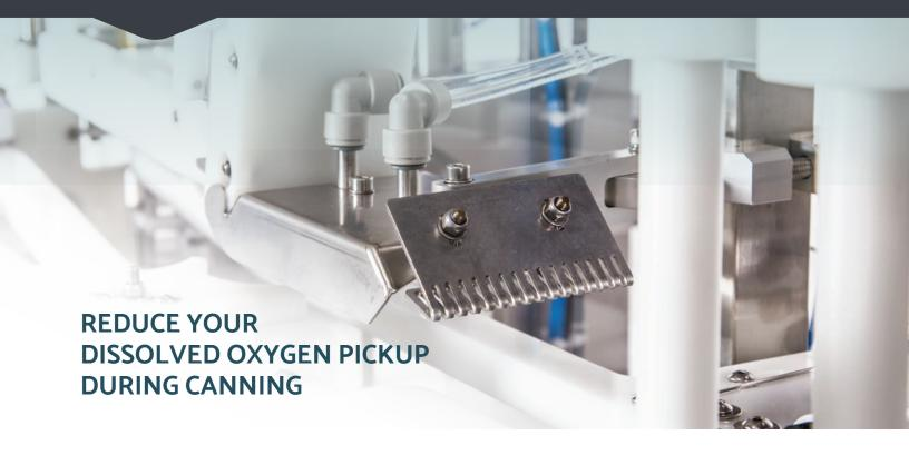
With adjustable underlid  $CO_2$  dispensing and a foam scraper, the D.O. Buster<sup>TM</sup>  $CO_2$  Tunnel preserves product quality by minimizing dissolved oxygen between fill and lid placement.
